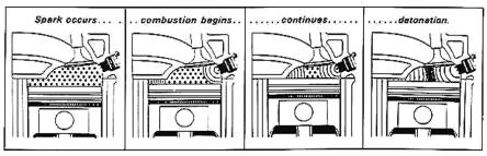
The damage resulting from preignition and detonation usually means that the piston must be replaced. For this reason, it is important to know the conditions that contribute to detonation and preignition so they may be prevented. The chart below is an outline of the principal causes of abnormal combustion.
