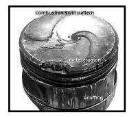
mixture does not all burn at the same instant. The flame front moves rapidly, but with controlled speed, from the point of the spark to the outer edges of the combustion chamber. Abnormal combustion occurs when the fuel burns in a different manner from that described above.
